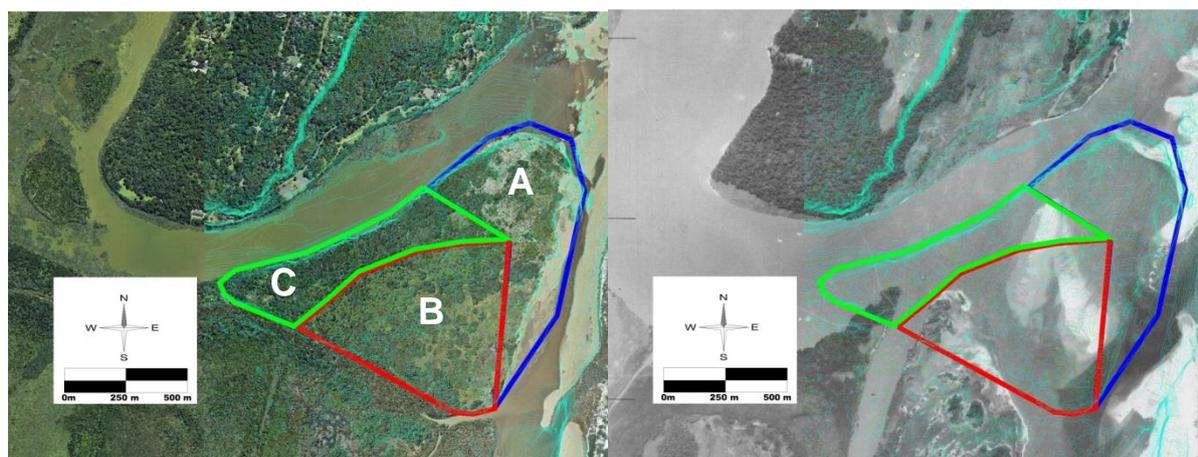
**Figure 4.5.** Approach recommended for the phased removal of dredge spoil that had been historically dumped between the uMfolozi mouth and the St Lucia Narrows. The “Combined mouth” scenario evaluated in the GEF study (Clark et al. 2014) corresponded with the removal of dredge spoil in area A (diagram on left) while in the “Reference” state it was assumed that sediment had been removed from all three compartments as per the 1937 configuration on the right.
