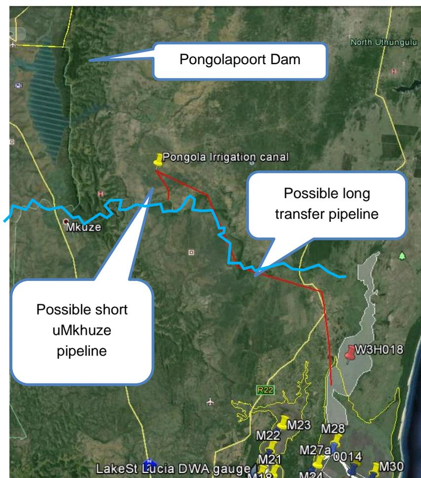
**Figure 9.14 Proposed water transfer pipeline routes from the Pongola irrigation canal to the uMkhuze River.**
