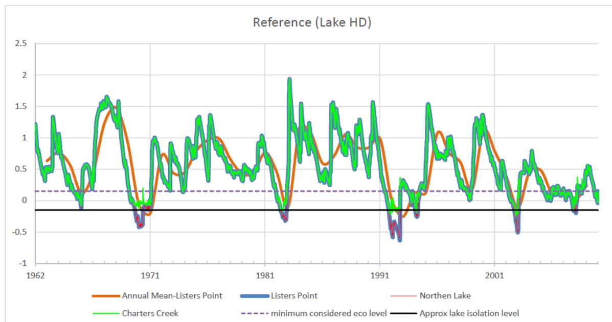
**Figure 9.3 Simulated water levels in the Lake with critical Lake levels for the Reference scenario (m MSL)**
