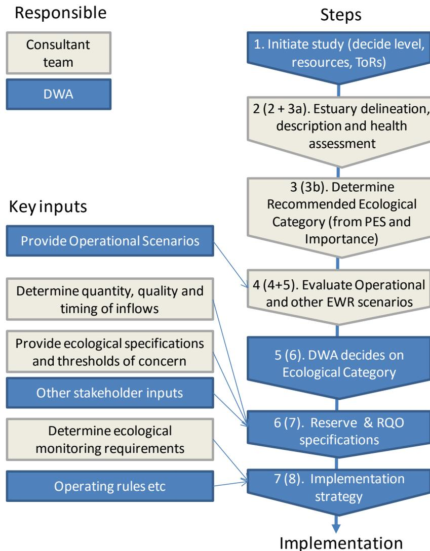
**Figure 3.1. Procedures for determination of the preliminary Reserve for estuaries, giving Version 3 step numbers and former step numbers in parentheses (Source: DWA 2012).**
