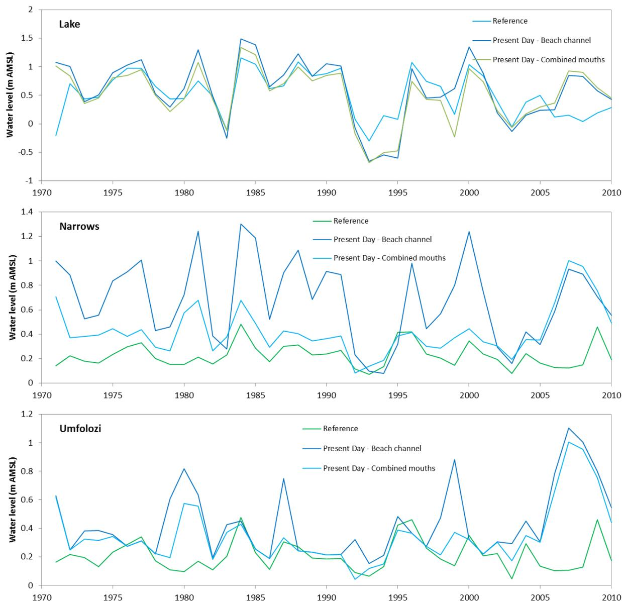
**Figure 4.23.** Mean water level in the Lakes, Narrows and uMfolozi for the Reference and Present Day. Note that present-day conditions have been modelled as two separate scenarios – Mouth A with the existing beach channel in place and Mouth B after Phase 1 of the dredge spoil removal process has been completed.
