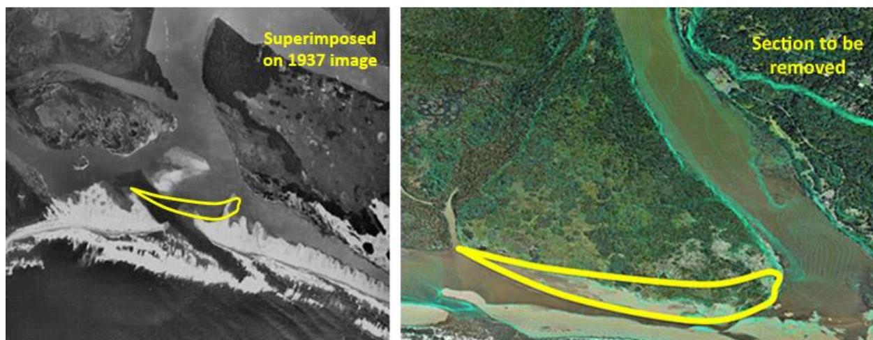
**Figure 4.4.** The mouth of the Lake St Lucia system in 1937 (left) and as it is at present (2013, right). The 2013 photograph shows the dredge spoil material that was placed in the river course from the 1950s for a period to try and separate the uMfolozi River from Lake St Lucia. The yellow boundary shows the first portion of dredge spoil that will be removed as part of Phase 1 of the restoration action.
