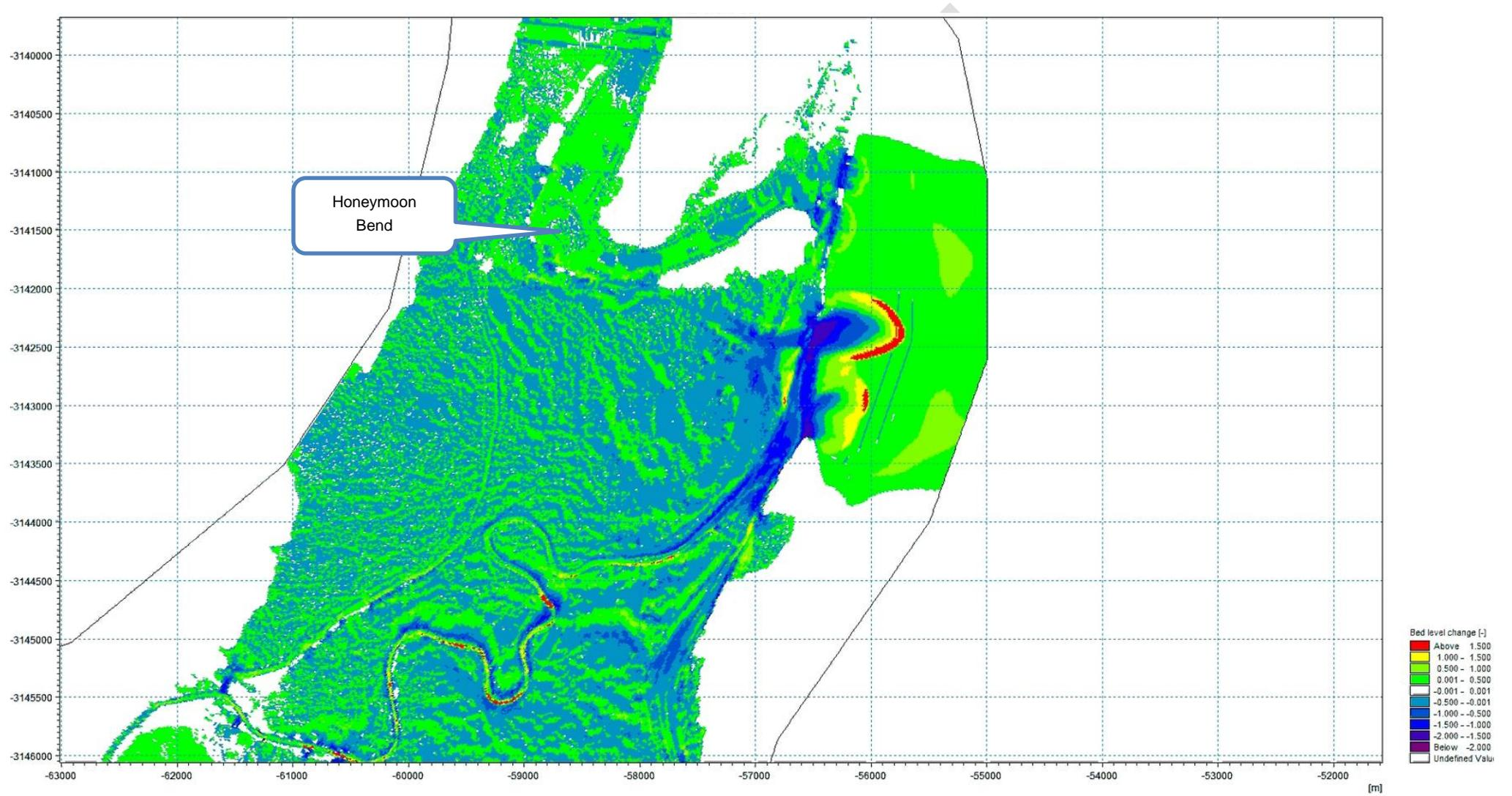
Figure 4.19. Model simulations showing change in bed level around Honeymoon Bend following a 1:100 year flood (Source: Basson *et al.* 2014).
