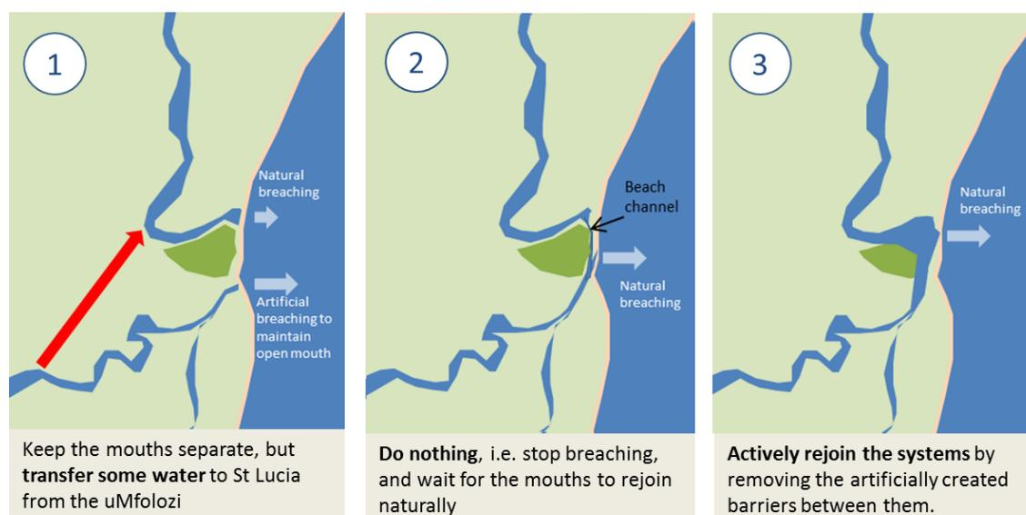
**Figure 4.2.** Schematic diagram of the three options considered in this study to restore the hydrodynamic functioning of the system (Source: Clark *et al.* 2014b).
